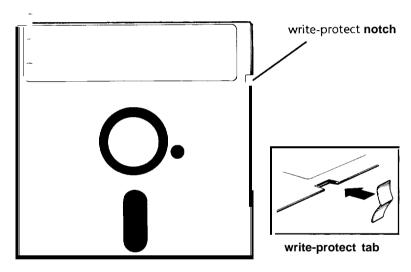
To remove the write protection, peel off the write-protect tab.
